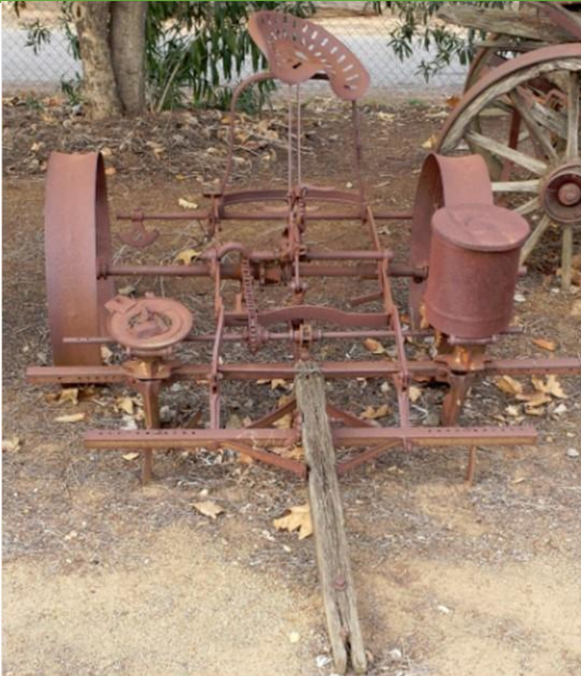
The adjustable Row Seeder designed in the 1880s, is pulled by a two horse team. The hoppers drop corn seed in a straight line into the plowed furrows. The wide flat wheels then push the loose dirt over the seeds. One hopper has been lost from this old machine. Fallbrook Historical Society
