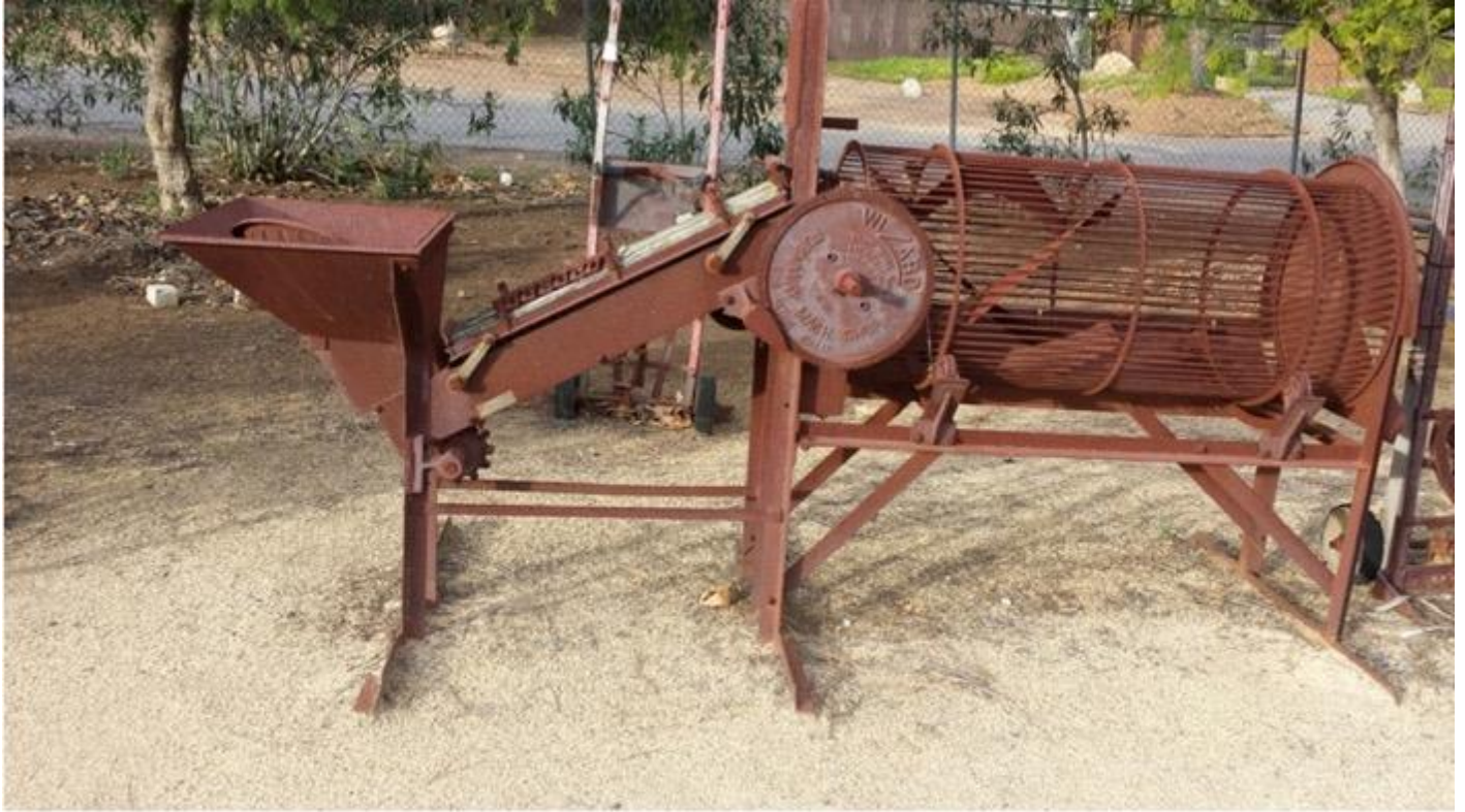
1939 Formway Wizard Walnut huller. Walnuts poured into the scoop were fed into the manually rotating cylinder. After the hulls cracked, walnuts fell into a tray placed below the cylinder. Fallbrook Historical Society
