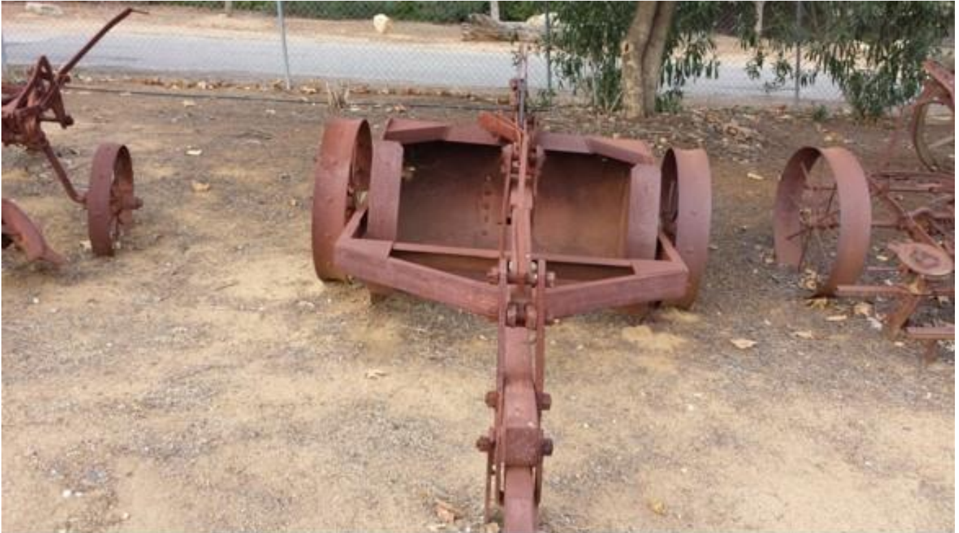
1882 Fresno Scraper a horse drawn earth scrapper used for constructing irrigation canals and ditches. Invented in 1882 & manufactured in Fresno by James Porteous, It was in high demand by farmers. Fallbrook Historical Society
